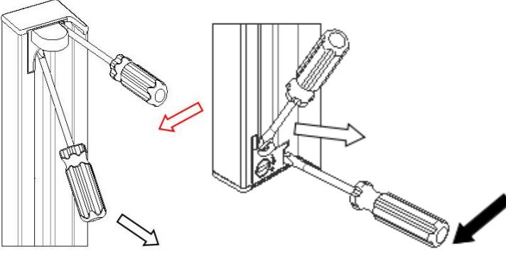
**Step2:** Insert a small flat-head screwdriver into the clip of the end cap. Pry off the clip and push out the guide rod. (All guide rod removal operations are the same.)
