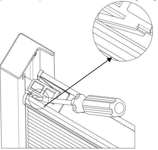
**Step3:** Remove the guide rod from the side channel.
