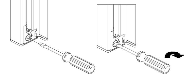
If the cord is over tightened, use a small flat-head screwdriver to pry up the bottom rail housing base from the notch. Meanwhile, insert another small flat-head screwdriver into the base from top to bottom to pull it out. Then, insert the flat-head screwdriver in the slot and press the rotating shaft, and then rotate anticlockwise to loosen the cord. Press back the rotating shaft and install the housing base back to the side channel.
