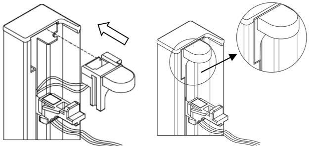
\*It's suggested to install the left bottom guide rod and housing base first, then the right bottom guide rod and housing base, then the left top guide rod and housing base and last the right top guide rod and housing base
