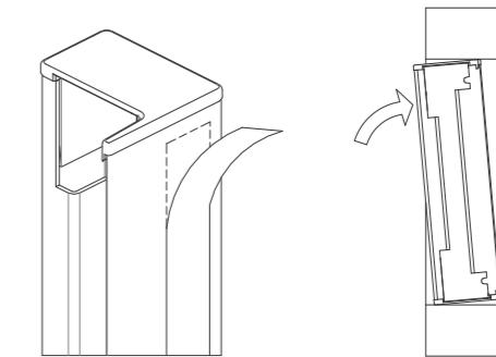
Notes: After the side channels are attached, do not pull the shade or side channels vertically outward for 48 hours.
